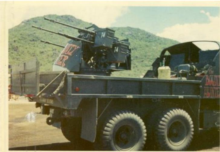
The M35A1 was a beast of a truck when equipped with heavy weapons, some crew served others manned by individuals. Examples of armaments include the Quad-50, four M2 Browning Machine Guns, M60 Squad Automatic Weapon (SAW), Grenade Launcher, and even the M134 Mini Gun.
