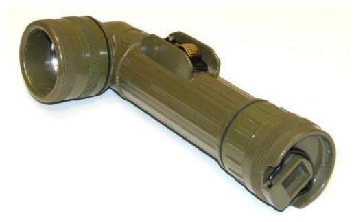
Flashlight model MX-991/U has been in production and issuance to the US Army and US Marines since 1963 after extensive testing and final approval of design. Keeping the iconic shape, improved features that would be implemented over the successive years included reliable gaskets, additional multi-color lens covers, stronger body material, and a switch guard to prevent accidental-lighting.
